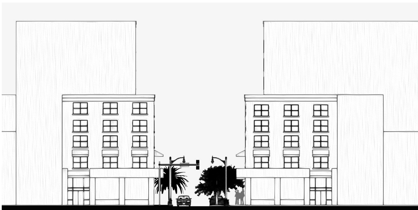
Figure 3.7: Core Street Section (50' ROW)
