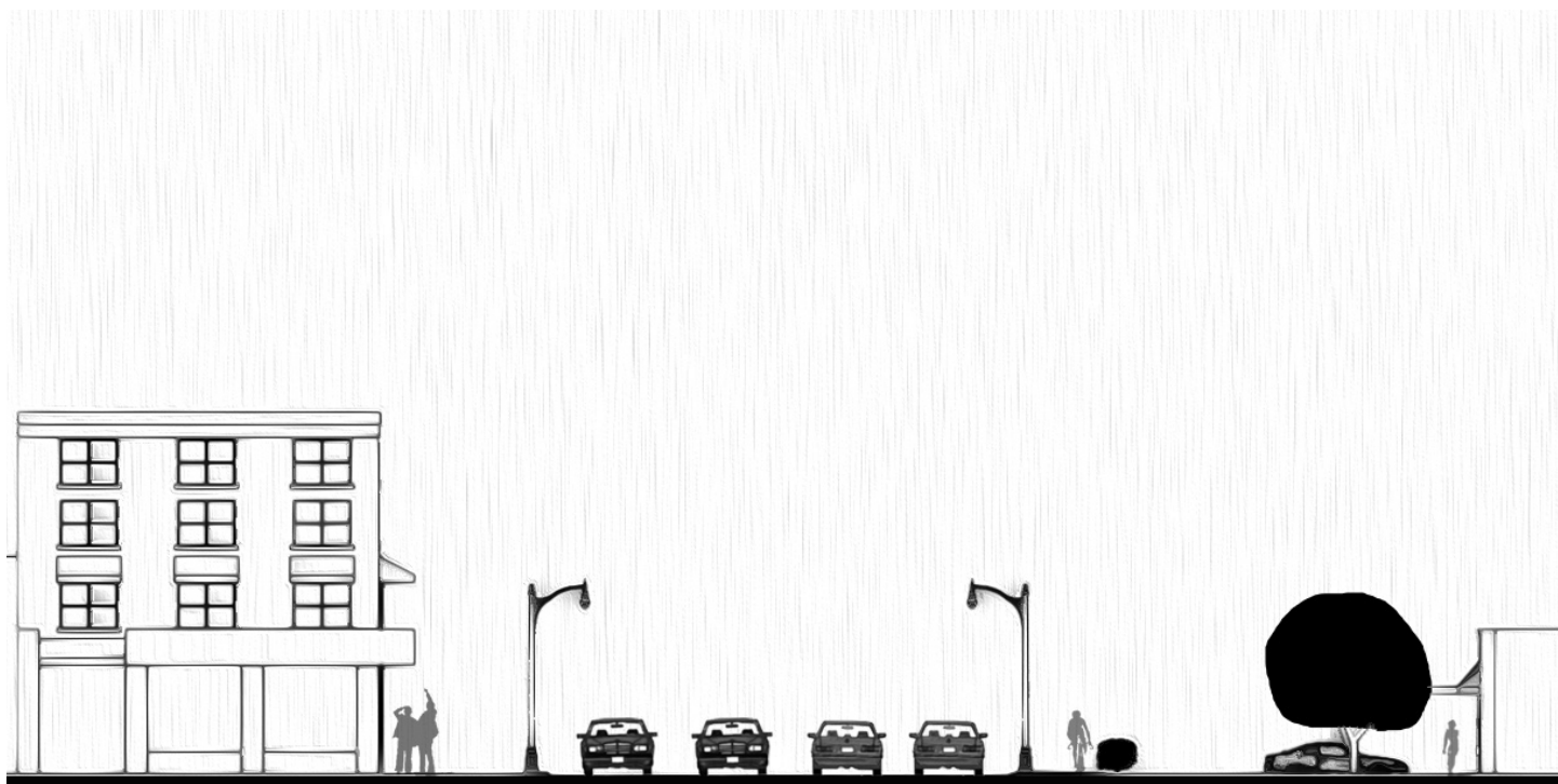
Figure 3.15: Thoroughfare Section (100' ROW)
