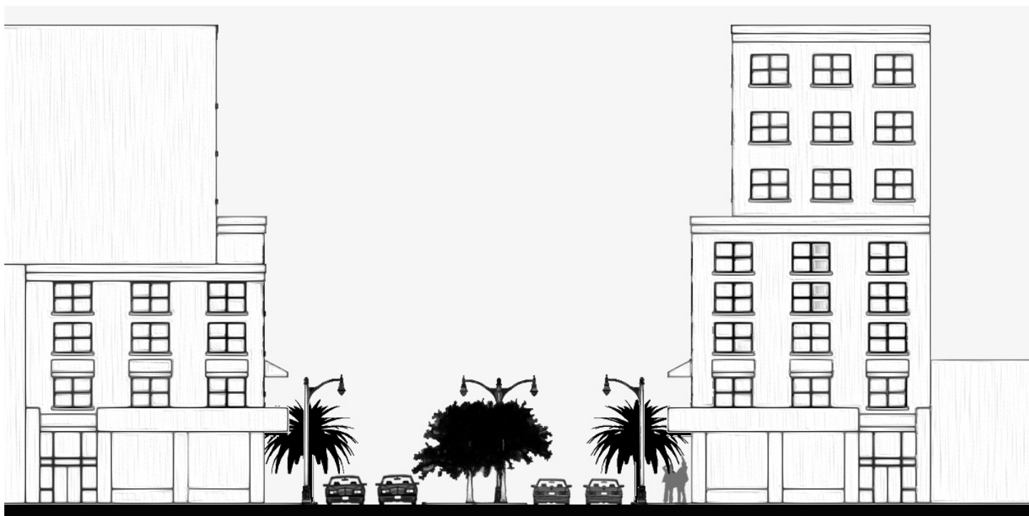
Figure 3.9: Core Street Section (SR 40, 90' ROW)
