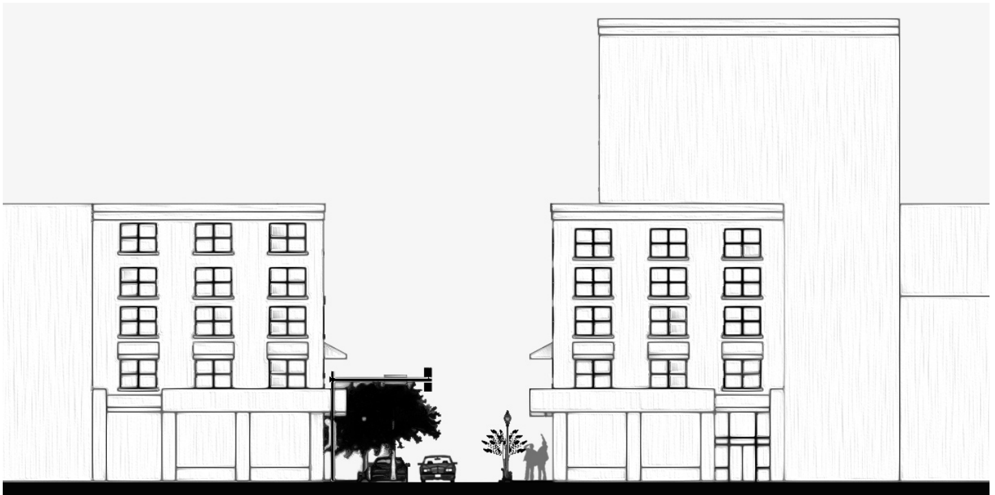
Figure 3.11: Standard Street Section (50' ROW)
